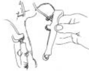
3.6 Trigger/assembly (13) can now be lifted out.
